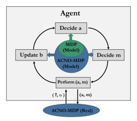
Figure 3: The control-loop for solving ACNO-MDPs using the *act-then-measure* heuristic. At each time step, a control action a is chosen according to the current belief state b, as though it is a belief over MDP states. Then, a measurement m is picked without ignoring the state uncertainty, (a, m) is executed, and the belief state b is updated accordingly.
